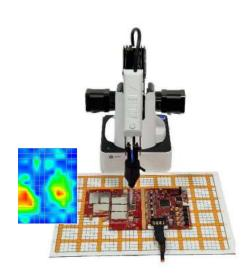
Using Handheld probes to identify and resolve EMC/EMI issue testing has never been this accurate. 3D Precision Technology used to assist high density board designers to use off the shelf hand-held probes and/or Y.I.C. Technologies probes and visualise the root causes of potential EMC and EMI problems during pre and post EMC compliance testing.
